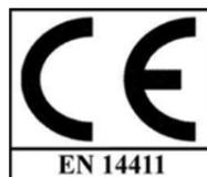
The CE ("European Conformity") mark certifies compliance of the product with the safety requirements of Community Directive 89/106/EEC and the mandatory requirements for construction materials, both in terms of health of users and safety. All items we produce feature the CE mark, clearly printed on the package. All CE compliance certificates are available for all series on our web site in Italian, English, French and German (upon demand in other languages of the European Union).
